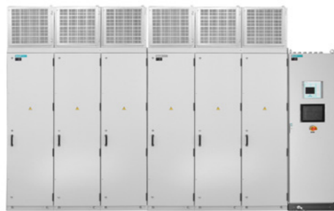
Type of converter: Current Source Inverter with Load Commutated inverter (LCI) technology Application: synchronous machines Voltage class: 3-15 kV Power range: up to 100 MW
