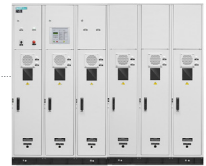
Medium voltage soft starters Type of soft starter: Current Source Inverter with Load Commutated inverter (LCI) technology Voltage class: 3-15 kV Power range: up to 220 MW
